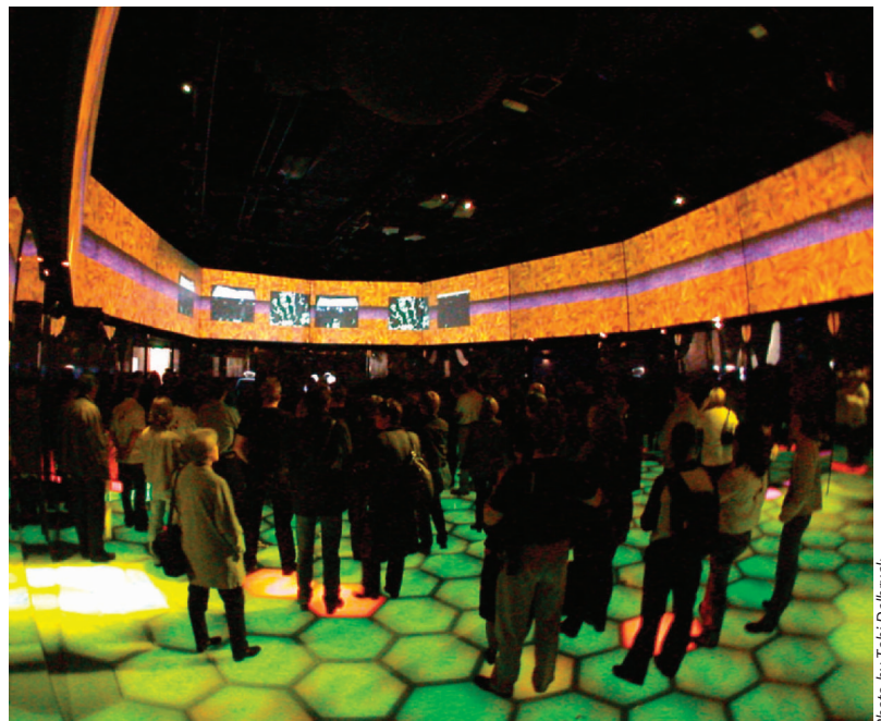
Figure 2. The Ada main space (from Figure 1c). The hexagonal floor tiles are pressure sensitive and display colored patterns dependent on Ada's behavior modes and on visitor interactions. The walls are made of semitransparent mirrors and allow visitors in the voyeur corridor (see Figure 1b) to view what happens inside Ada. Above the mirrors a circular projection screen displays real-time animated graphics that, similar to the music, represent Ada's current behavior and emotional state.
